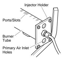
Figure 30 - Injector Holder On Outlet Burner Tube
